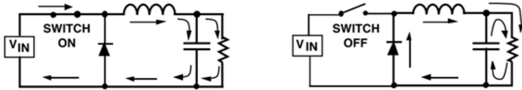
Figure 14: Buck Regulator Switching Current Flow Paths ( Texas Instruments )
